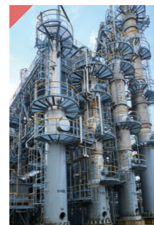
7 Stabilizer Column Heats and regulates the vapor pressure of oil to allow safe transport by Tanker trucks.
