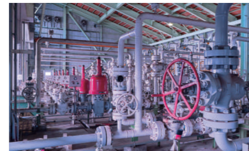
1 Inlet Manifold Collects fluids (natural gas, oil, etc.) sent from the wellhead facilities around the plant.
