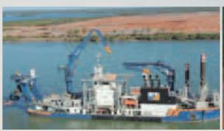
Dredging work in the Port of Darwin To secure the route to be taken by tankers and other vessels, a dredger is deepening the sea floor in the area around the construction site in the bay. The photo shows the dredger Athena.
