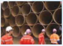
Sections of the 42-inch diameter steel pipes that have been transported to Malaysia for coating
