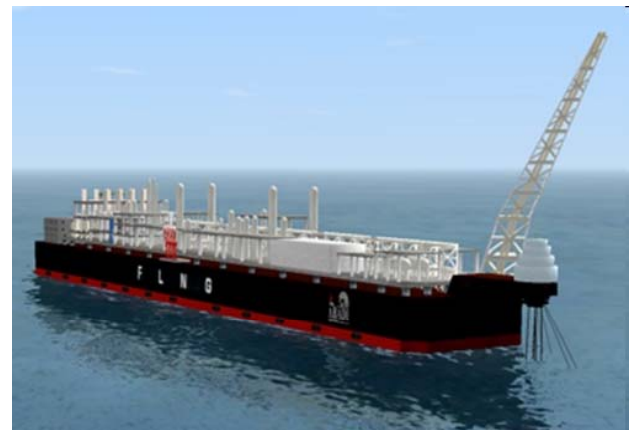
FLNG 3D Imaga Hull Size: 500m length × 82m width
